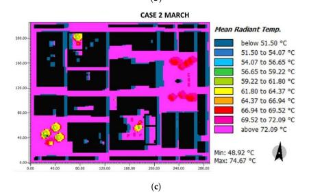
Figure 13. Results maps for radiant mean temperature for March at 15:00: (a) base case, (b) case 1, and (c) case 2.
