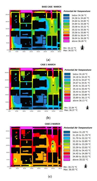
**Figure 11.** Results maps for potential air temperature for March at 15:00: (**a**) base case, (**b**) case 1, and (**c**) case 2.
