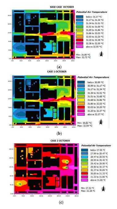
Figure 12. Results maps for potential air temperature for October at 15:00: (a) base case, (b) case 1, and (c) case 2.
