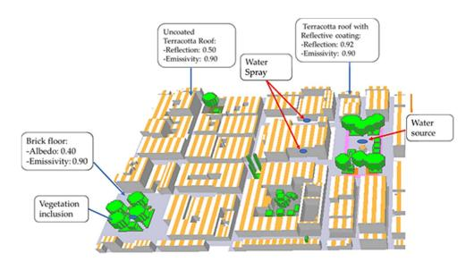
Figure 9. Schematic of case 2 developed in Envi-met.
