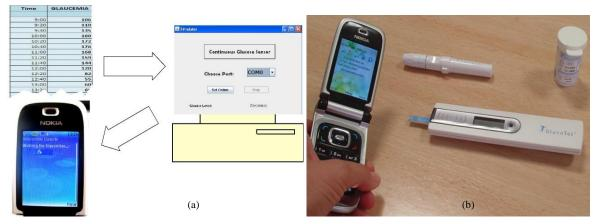
Figure 6. (a). Continuos glucose sensor simulation, (b). Communication between mobile phone and glucometer
